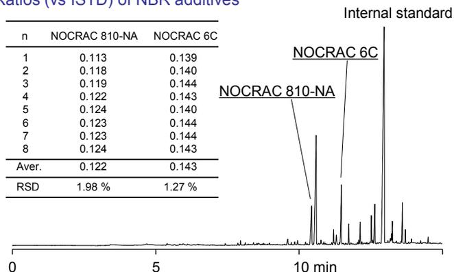
Fig. 2 Chromatogram for Zone A by (TD)-GC/MS analysis
