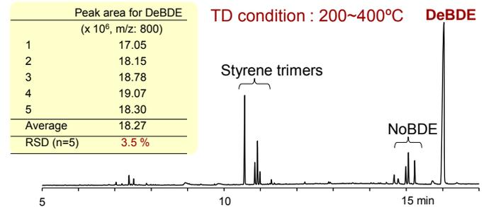
Fig. 2 Chromatogram of waste plastic obtained by (TD)-GC/MS
