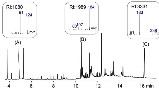
(b) Chromatogram of *p*-(*p*-toluene sulfonylamido) diphenylamine stored in MS library
