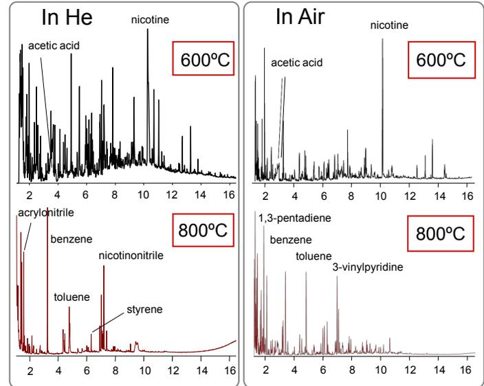
**Fig. 1** Pyrograms of tobacco obtained at 600°C and 800°C under air and helium atmosphere
