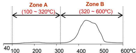
Fig. 1 EGA Profile of Polypropylene + Nylon
