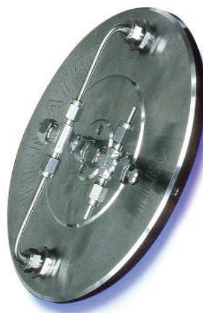
Figure 5: The Field and Laboratory Emission Cell (FLEC) for material emissions testing.
