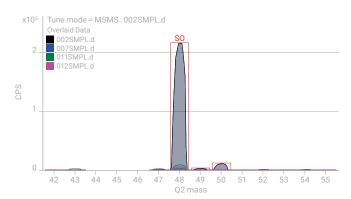
With MS/MS, Q1 rejects the Ca\*, Ti\* and C\* ions, so the SO\* product ions are measured accurately and consistently, free from overlap.
