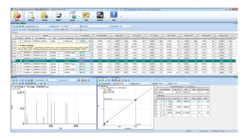
ICP-MS MassHunter Data Analysis pane, showing interactive batch table, outlier flags, current sample spectrum, and calibration summary.
