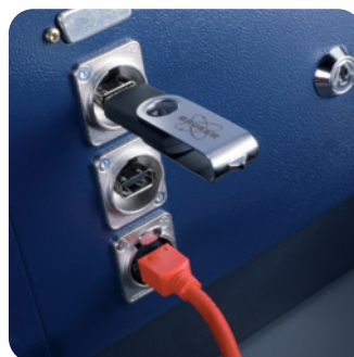
USB and Ethernet connectors
