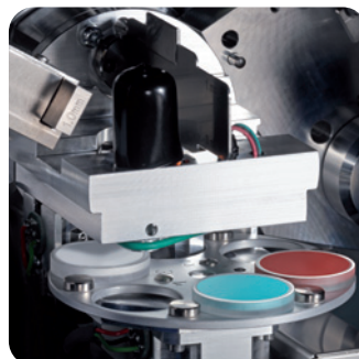
Six position sample changer
