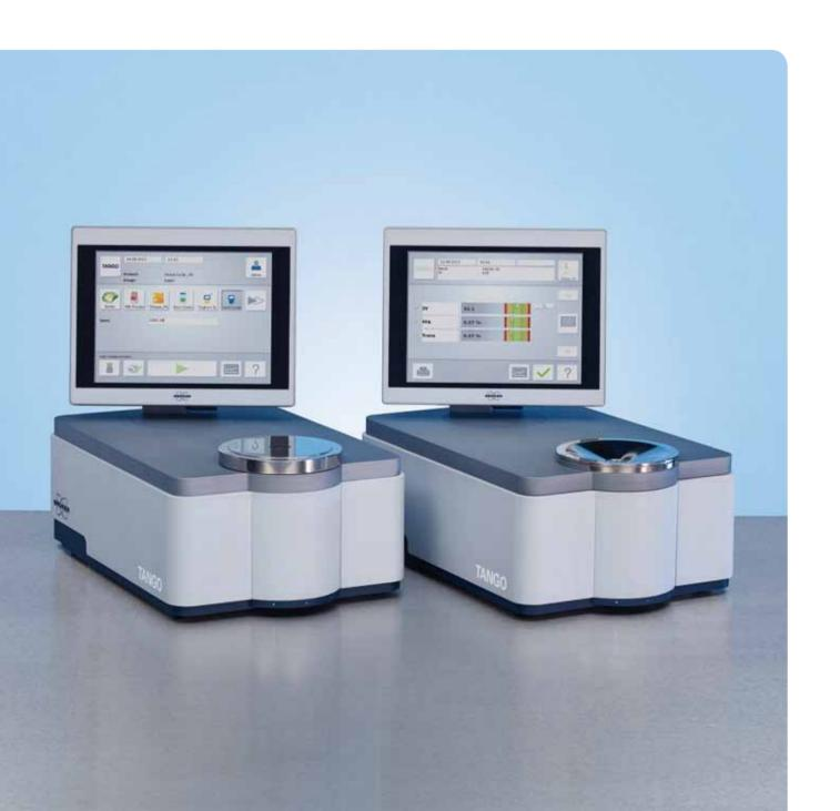
Select the TANGO you need. The reflection analyzer for solids or the transmission analyzer for liquids. With or without integrated PC and monitor.
