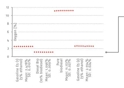
Reproducibility of oxygen concentration measurement of liquid fuel samples using rapid OXY cube equipped with vario liquid sampler (VLS).
