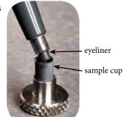
The *eyeliner* is placed directly into the sample cup and analyzed directly; there is *no sample prep*.
