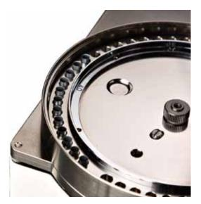
Up to 48 samples can be analyzed. When performing multiple analyses on a single sample, the sample is held at near-ambient temperature between analyses. The sample path has one isolation valve and two magnetic cup positioning valves which are always at ambient temperature.
