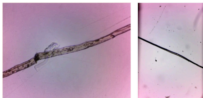
Figure 4: Left image shows video micrograph of fiber in compression cell. Right image shows video micrograph of fiber viewed through the ATR crystal.
