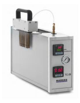
The TC-20 uses a flow of clean nitrogen to condition or dry-purge up to 20 industry-standard stainless steel, inert-coated or glass sorbent tubes at temperatures up to 400°C.
