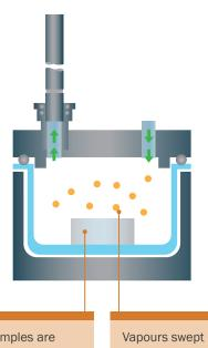
Samples are Vapours swept placed straight from the entire sample are chambers. Vapours swept from the entire sample are collected.
