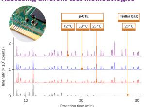
Quick investigations of how emission profiles vary under different conditions are easily conducted using the μ-CTE. This example shows the detection of residual solvents in **printed circuit boards**.
