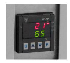
Each chamber lid is closed, a flow of gas (air or nitrogen) is applied, and the temperature selected – from ambient up to 120°C or 250°C depending on the model of µ-CTE chosen.
