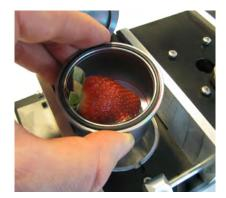
The sample is placed inside one of the chambers. Up to four or six samples can be accommodated, depending on the model of  $\mu\text{-CTE}$  chosen.
