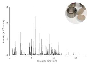
The µ-CTE is ideal for screening emissions from products such as flooring and **plasterboard**, for routine factory production control under the Construction Products Regulation (see prEN 16516).
