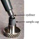
The *eyeliner* is placed directly into the sample cup and analyzed directly; there is *no sample prep*.
