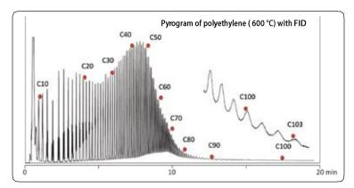
Precision and accuracy reflect the thermal homogeneity of the system thermal gradients between the 3030D and GC are eliminated by replacing the standard septum nut with one that fits snugly into the unique heat sink adapter at the bottom of the pyrolyzer. The effectiveness of this design is underscored by the C100 chromatogram.
