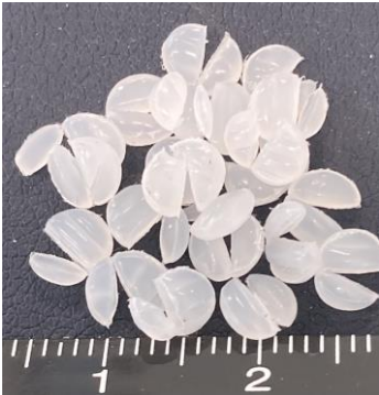
HDPE 0.48 g Pretreatment: Cut in half with nippers
