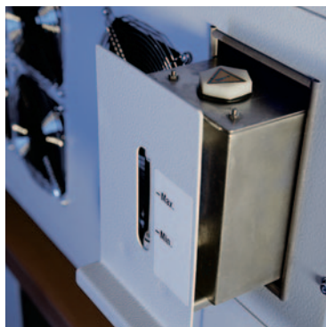
Internal water chiller
