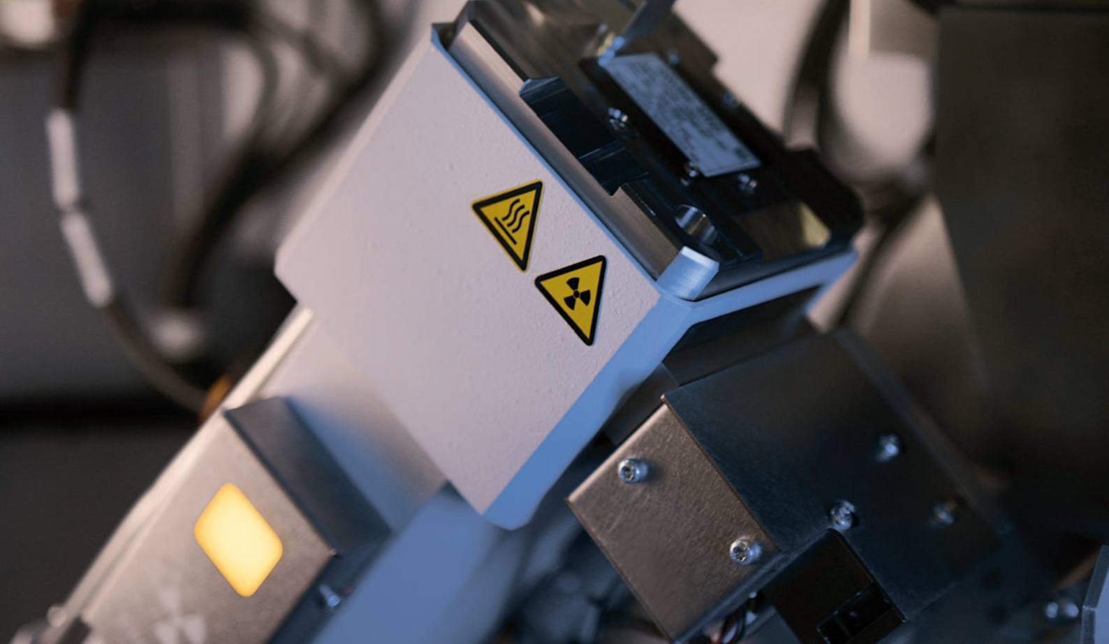
X-ray source power options: 540 W, 600 W, or 1.2 kW
