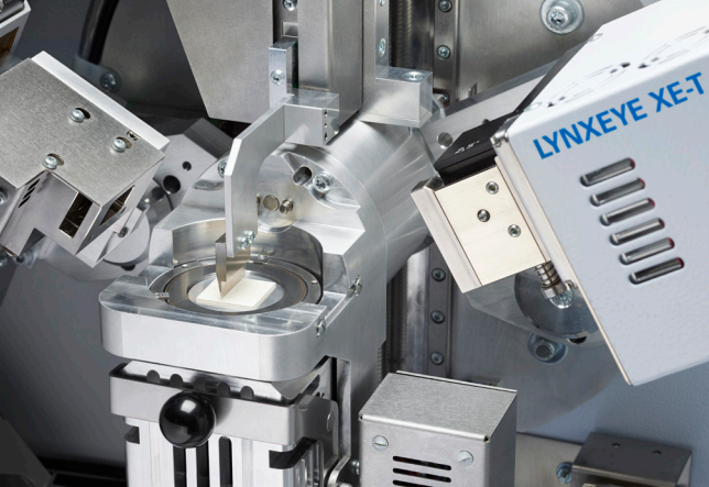
Figure 2 D6 PHASER equipped for Dynamic Beam Optimization (DBO) with Variable Divergence Slit (VDS), Motorized Air Scatter Screen (MASS) and LYNXEYE XE-T detector.
